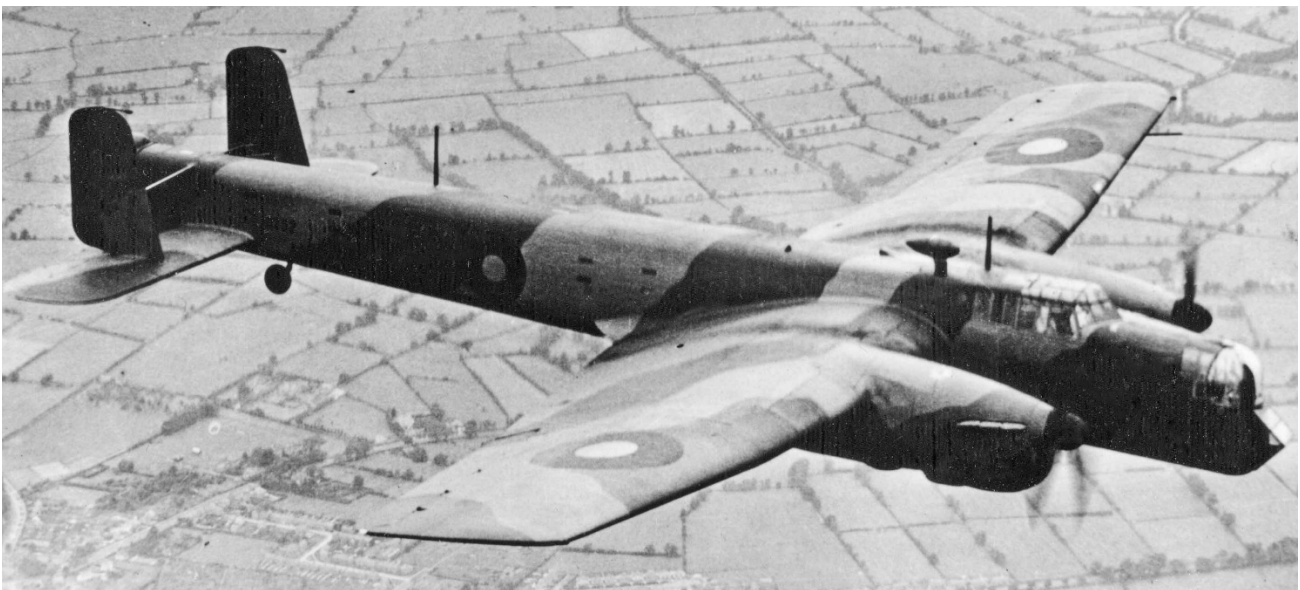
An air-to-air photograph of an AW38 Whitley showing its characteristic nose-down attitude in flight.
